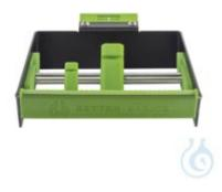
The donor for adhesive tape or labeling band was developed to record up to 6 rollers with a core hole diameter of approx. 25 mm (1 inch) or approx. 76 mm (3 inches) with a total width of up to 160 mm.
